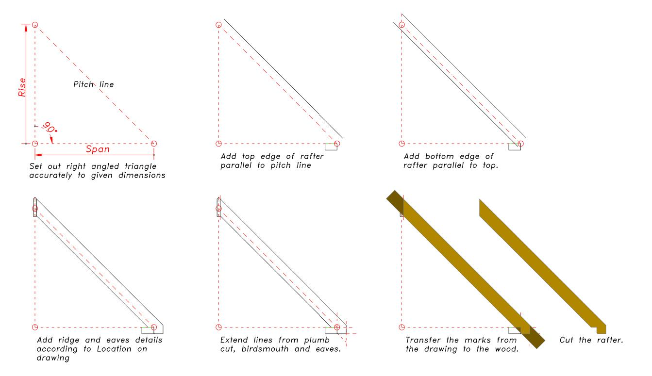
Setting out and marking the COMMON RAFTER.
